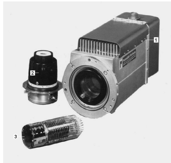
Figure 3. Detector: (1) Socket, (2) cooler and (3) photomultiplier (PMT).
