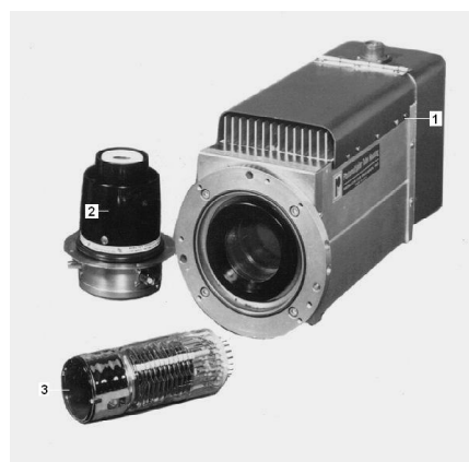
Figure 3. Detector: (1) Socket, (2) cooler and (3) photomultiplier (PMT).
