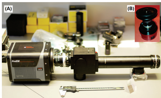
Fig. 9. New instruments at KHO 2015. Panel (A): Meridian Imaging Svalbard Spectrograph (MISS). Panel (B): The ZWO ASI174MC F/1.4 all-sky color camera.
