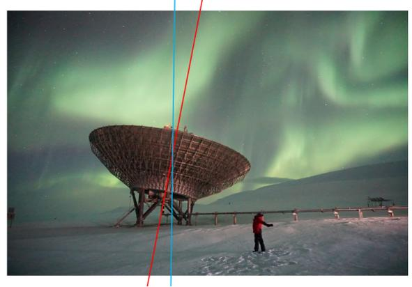
Figure 1.8: EISCAT Svalbard radar, 42 meters fixed parabolic antenna aligned along the direction of the local geomagnetic field (red line). The blue line represent the local vertical. Credits: Katie Herlingshaw
