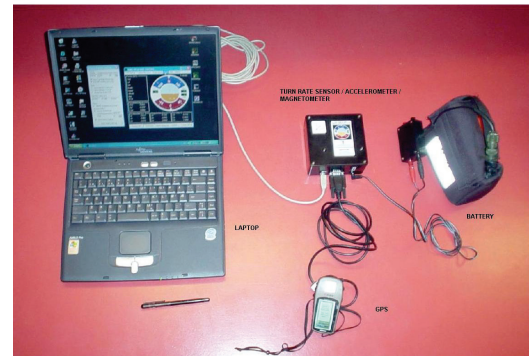
Figure 7.4. The GPS is linked to the laptop via a USB hub. The turn rate sensors / accelerometers / magnetometers are connected to the laptop with the same hub. The sensors are powered by +12VDC battery.
