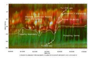
Fig. 2. Meridian Scanning Photometer (MSP) from the Auroral Station in Adventdalen 25 January 1995. The red, green and blue colors represents the auroral emissions 6300 [OI], 5577Å [OI] and 4278Å  $[N_2^+ 1NG]$ , respectively (Lorentzen et al., 1996).
