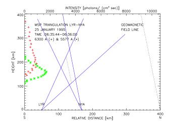
**Fig. 3.** The volume emission rate as a function of altitude 25 January 1995 from Ny-Ålesund (NYA) and the Auroral Station in Adventdalen (LYR). The [OI] 6300Å is plotted as (+) and the [OI] 5577Å as (\*).
