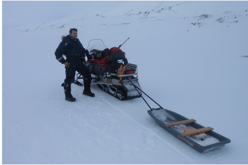
Figure 8: GPR used in Longyearbreen and SFS. The sledge pulled by the snow scooter allows to cover large areas in a short time.
