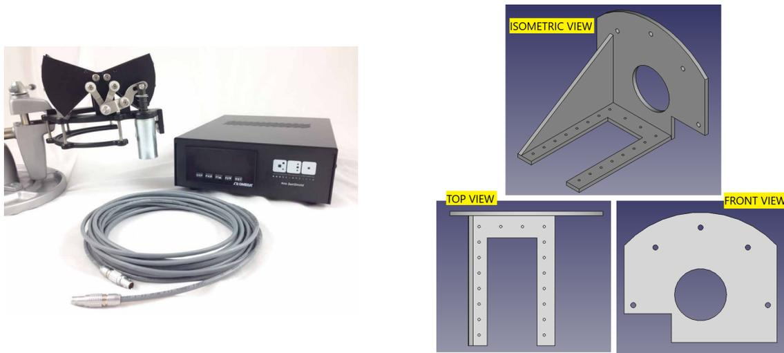
**Figure 4.14:** Left: Equipment required to operate the SunShield [40] Right: Own Design Suggestion, 3-piece interlocking aluminium SunShield adapter fixed onto the breadboard. (Model created using FreeCAD)
